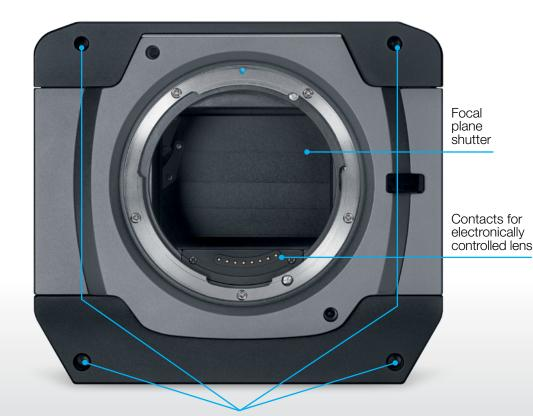
Screw threads for vertical mounting
