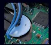
Advanced electronics, featuring analog front-end circuits to digitize the CCD signals, a dedicated printed circuit board with a low-noise design and patent-pending dual-output reading mechanism, result in a high signal quality with minimal noise and excellent linearity.
